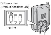
You can set the following functions by using the DIP switch 1 to 3.
